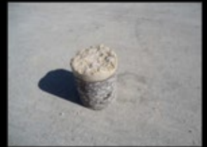
The emulsion sprayed prime coat- Base course core sample well bonded with sub base
