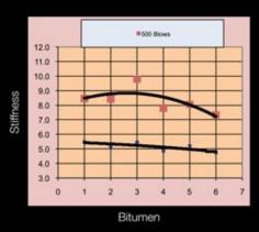
If we look at the above graphs we see that the flow is lowest at binder content 3. High flow can be associated with plasticity. Also binder content 3 exhibited the highest stiffness. Binder content 3 had 5.8% voids at 75 blows and 3.3% at 500 blows. From this we gave ourselves a voids target of approx 6% at 75 blows and a minimum of 3.0% at 500 blows. We have found that by using these parameters our asphalt has resisted rutting extremely well.
