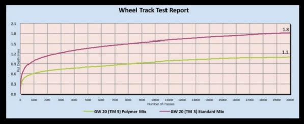
After determining the best method of maximising the performance of conventional asphalt, we looked to see how we could improve on this by adding a polymer modifier to the bitumen.
